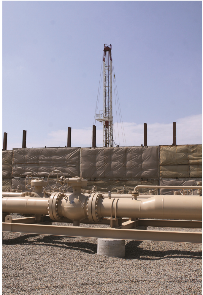
Local jurisdictions can require nuisance mitigation measures, such as these padded sound barriers, to reduce the negative impacts of oil and gas development on the community. Photo © Trudy E. Bell.
