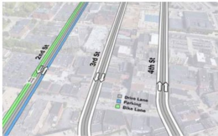
Scenario C: Remove parking on both sides of 3rd and 4th Streets to expand sidewalks to 25 to 30 feet wide
