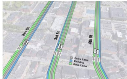
Scenario D: One-way pairs on 3rd and 4th become to two-way traffic to encourage commerce, long truck and bus movements, and bicycling-pedestrian safety and mobility
