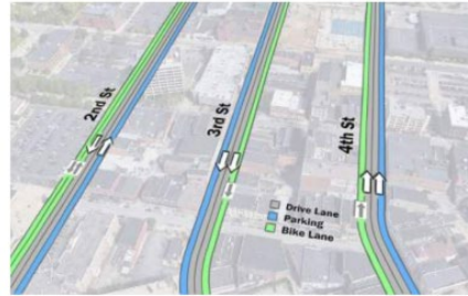
Scenario B: One-way bike lane on left hand side of 3rd and 4th Streets, requiring removal of parking from one side
