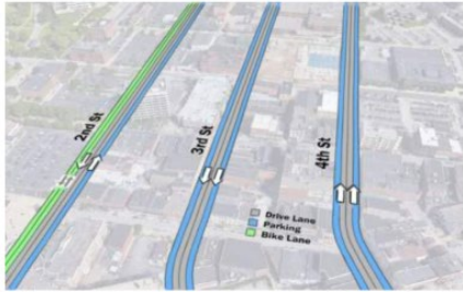
Scenario A: 2nd Street Cycletrack with no facilities on 3rd and 4th Streets
