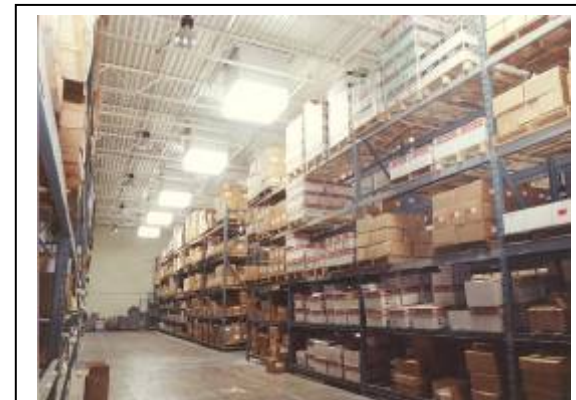
In the daytime, natural daylight can effectively light large indoor spaces such as this warehouse.
