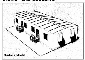
Collected point cloud data will be edited and modeled using computer aided design (CAD) software to develop surfaces representing the exterior building shell, fenestration, and architectural features. Outlying data points recorded during the scan (i.e., noise) and miscellaneous objects near the buildings that are recorded (i.e., artifacts) will be removed. After the data is cleaned and only those points that represent the buildings remain, a digital model will be developed.
