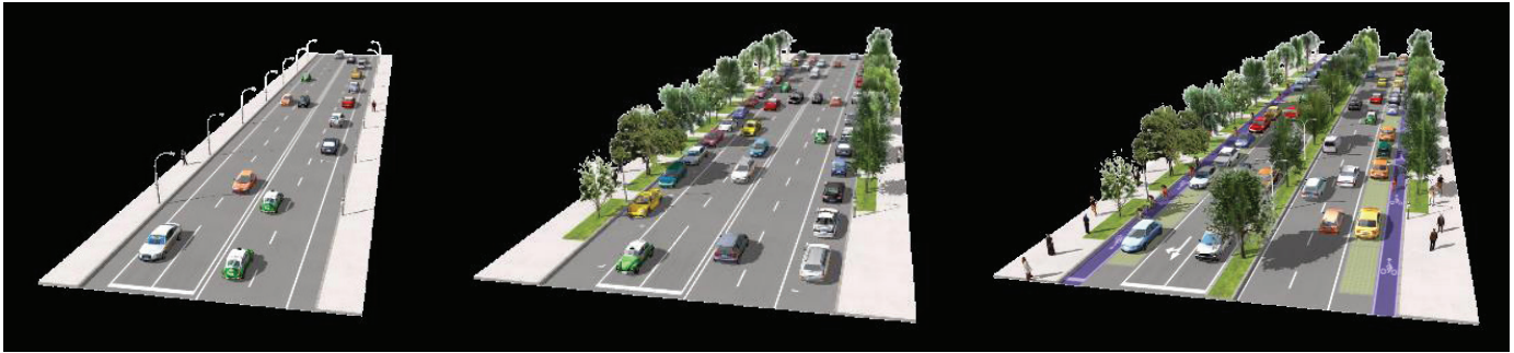
Figure 2: Using CityEngine’s complete streets rule , a planner can optimize a street scene across multiple variables such as walkability, bikeability, transit, carbon sequestration, and stormwater infiltration by changing parameters. Courtesy Esri.
