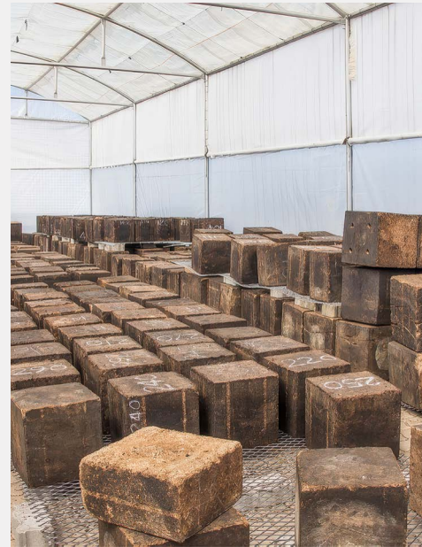
“Mycoblocks,” bricks made from local mushrooms, are a potential construction material for affordable housing in Namibia and other countries. Photo courtesy of MycoHAB.
