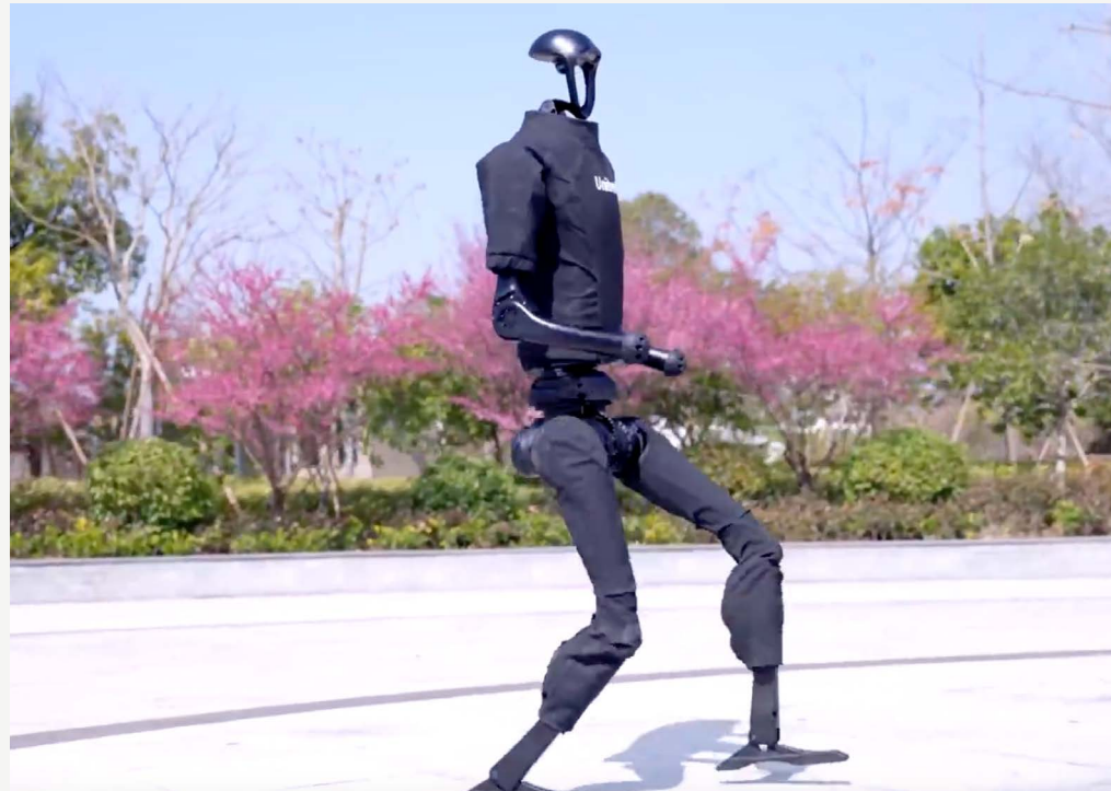
Advances in humanoid robot technology include the Chinese company Unitree's H1 robot, which in March 2024 broke the humanoid robot running speed record by reaching 7.4 miles per hour. Photo from Unitree video.
