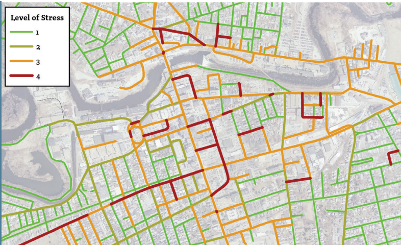
The Level of Traffic Stress street map displaying the walkability of streets in Nashua, New Hampshire.
