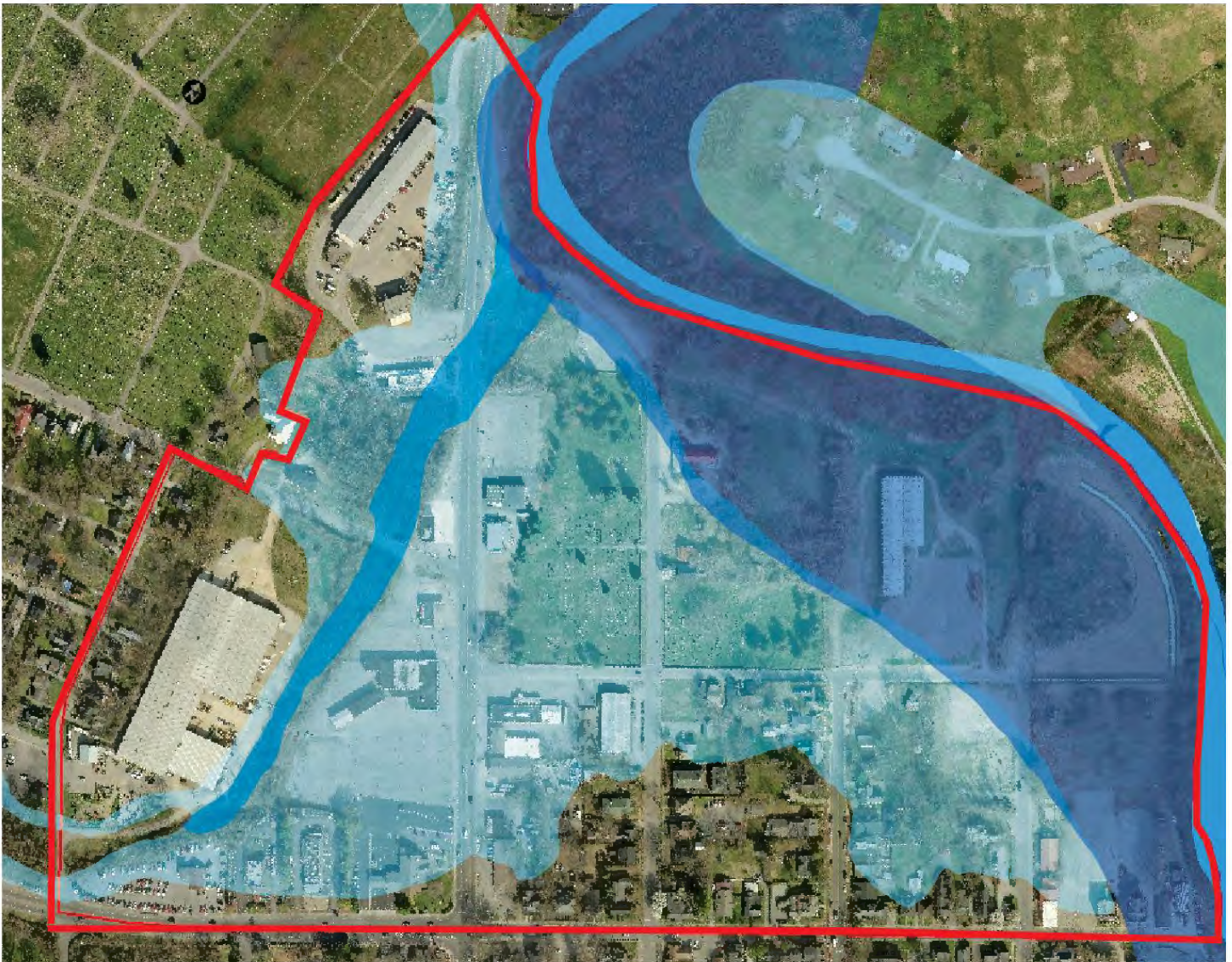
Diagram of the floodway and flood fringe areas
