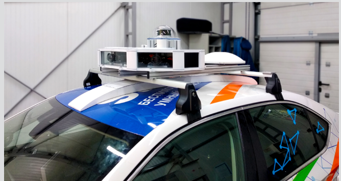
Figure 3. Vehicle-mounted Lidar equipment can be used to collect accessibility data (Alena Nesterova/Wikimedia (CC BY-SA 4.0))
