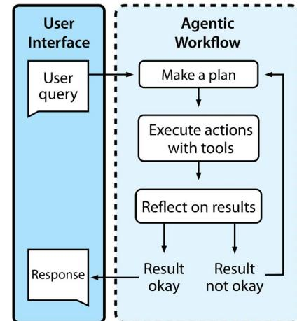
*Agentic AI systems are able to plan, execute actions, reflect on results, and modify their actions if needed. Illustration adapted from [Weaviate](#).*
