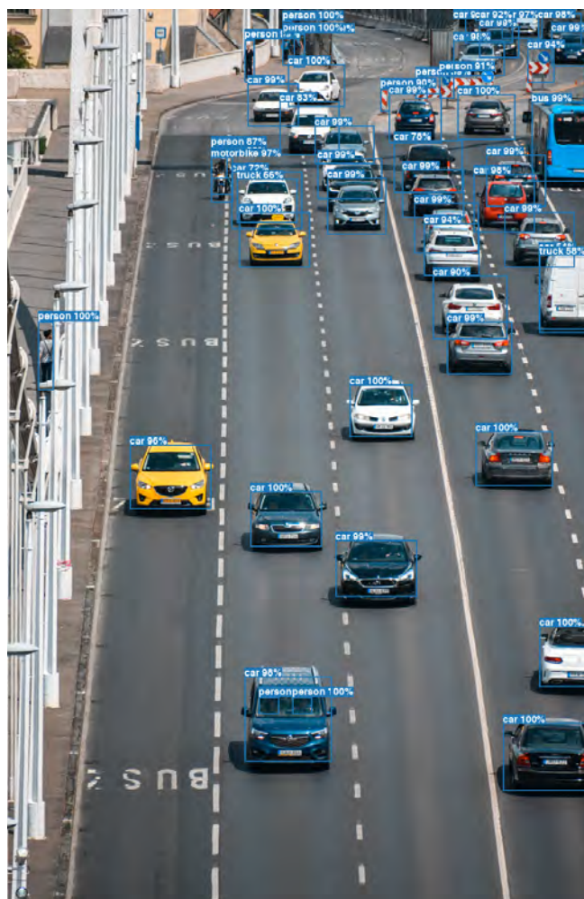
Figure 2.11. “ Bounding boxes ” applied by computer vision to identify different types of vehicles on a roadway (Photo by Keszthelyi Timi/Unsplash; bounding boxes created using Online Object Detector )
