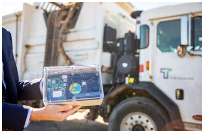
Figure 3.2. Cameras used on Tuscaloosa garbage trucks to collect conditions imagery (City of Tuscaloosa)
