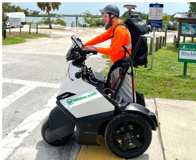
Figure 8.2. Data collection via Segway, with sensors mounted on the vehicle and lidar attached to the driver’s backpack (WGL Inc.)
