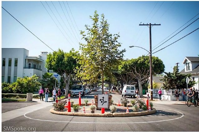
Figure 7.3. Pop-up roundabout in the Michigan Avenue Neighborhood Greenway in Santa Monica, California ( SMSpoke.org )
