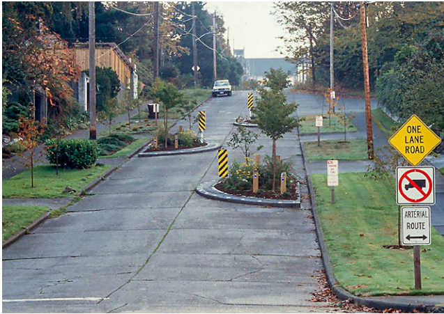
Figure 6.12. A chicane with three landscaped diverters requires drivers to perform two turning maneuvers on this otherwise straight street (Flickr/Richard Drdul CC BY-SA 2.0)
