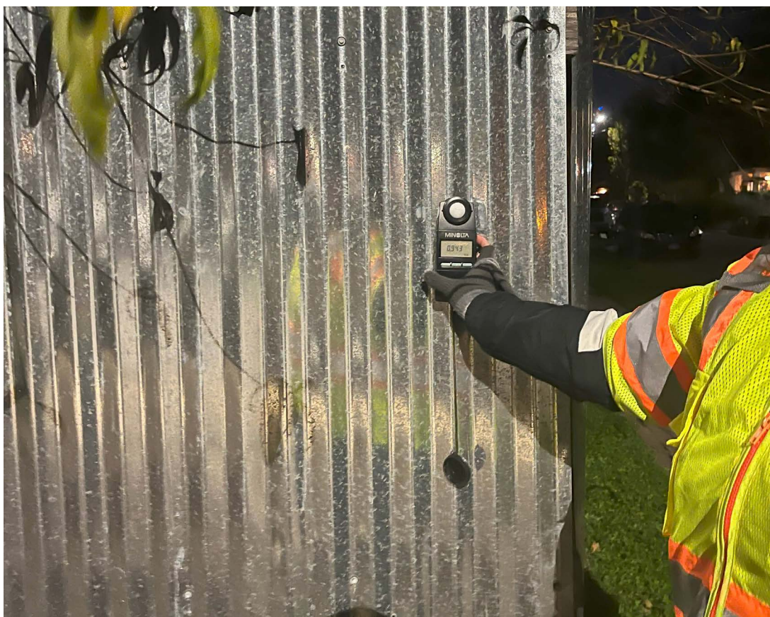
The author demonstrating proper use of an illuminance meter (Credit: Photo courtesy of Clanton & Associates)
