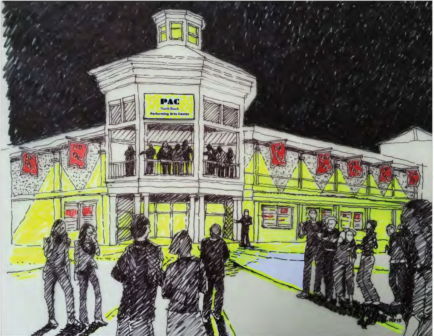
Figure 21: The rendering above shows what a Performing Arts Center could look like. A corner terrace faces the Chesapeake Bay as well as the activity along Fifth Street and Bay Avenue. The theater is on the second floor with the stage on the western end. Retail is on the first floor fronting both Bay and Fifth. A classroom is included on the first floor behind the retail. An apartment building with additional retail on the first floor would continue the western end of the Fifth Street block. (Drawing by Philip Franks, AICP, AIA)
