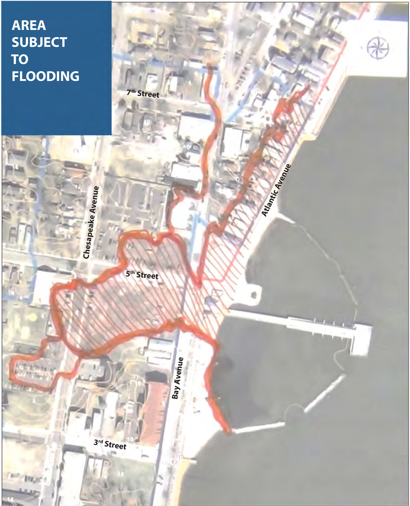
Figure 13: The red hash lines represent areas where flooding poses a threat. The scope of flood hazards is expected to increase with the effects of climate change. (Created by Philip Franks, AICP, AIA)
